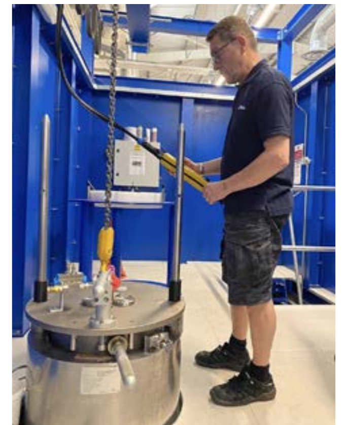
Trittech engineer carries out product pressure testing at the Ulverston site.
