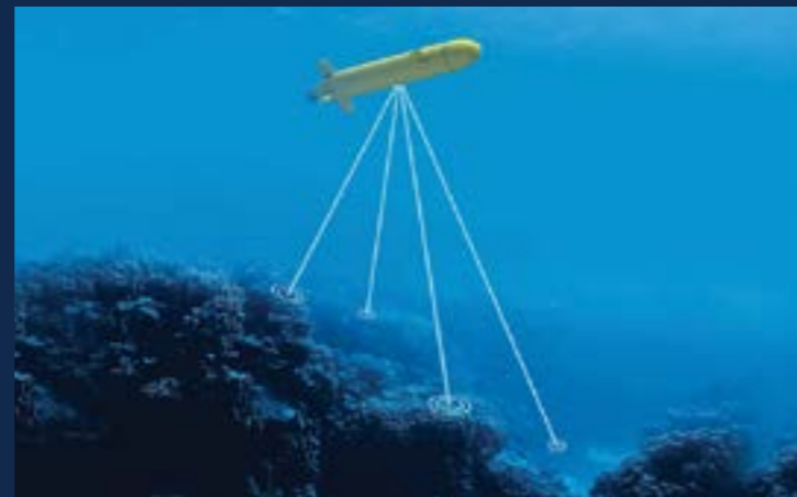
A DVL is an essential navigation tool for AUVs designed for long missions, or missions with high accuracy requirements.
